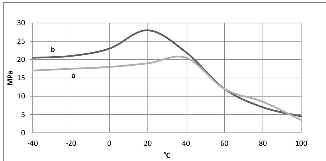
**Roller peel test (ISO 4578)**(typical average values) - Cure : 16 hours/40°C
